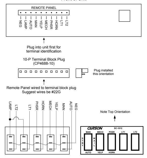
LT1 and LT2 Lighted Rocker Switches may control devices directly bypassing the unit.
